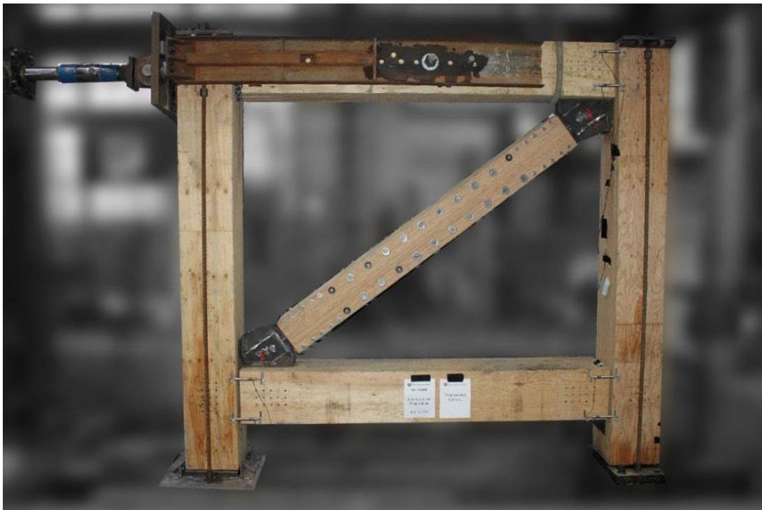
Test set up of the TBRB at University of Utah
