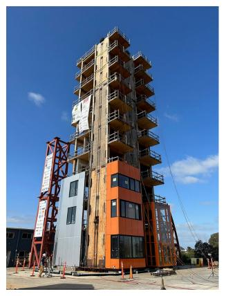
Post-tensioned rods run the full height of the 112-ft-tall specimen's mass-timber rocking walls. *Photo by Reid Zimmerman*
