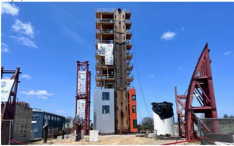
The shake-table specimen, at 112 ft in height, is the tallest mass timber frame ever tested for seismic resilience. *Photo by Rachel Judlowe*
