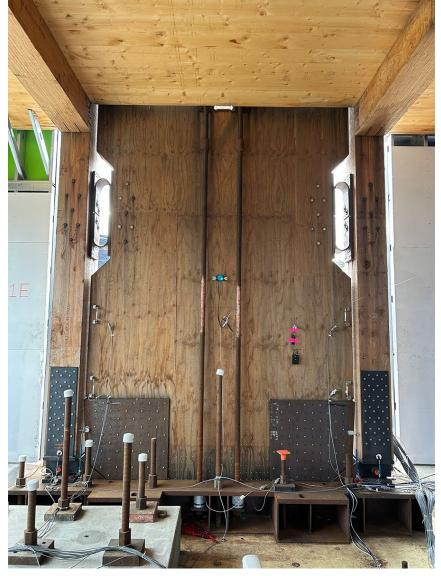
At the bottom of the walls, the rods anchor into the foundation. At the top of the walls, the rods attach to a steel "saddle" assembly which transfers the load from the threaded rods into the mass timber wall panels.
