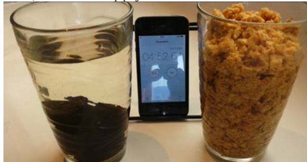
Arterran Advanced Fuels submerged in water (left) versus wood pellets submerged in water. Photo courtesy Arterran Renewables.
