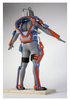
"Aegis gives extra power to the logging worker—the motor actuation will let them easily and safely finish the tasks," Lee told Core77. "Also, the exoskeleton provides protection from falling trees or limbs with the steel tubes will reduce the chances of getting injured. Since there aren't many parts on the lower body compared to the upper, it makes them able to move freely without struggling."
