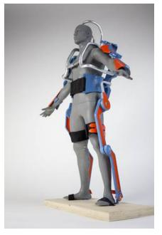
Aegis is designed to protect loggers from falling trees and branches, as well as injuries from chainsaws. It also assists with endurance – with motorized actuators in the limbs of the suit.
