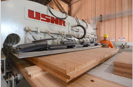
Manufacturing of cross-laminated timber. Photo: D.R. Johnson Wood Innovations
