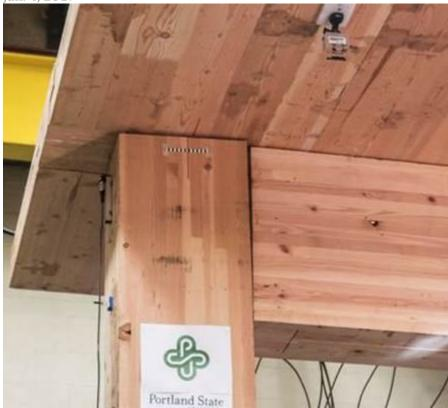
A wedge forms between pieces of timber that undergo an earthquake simulation at PSUs iSTAR Lab. Photo courtesy of SustainableLife
