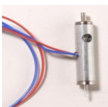
Figure. 4 Microfab piezoelectric droplet generator [12]. Figure. 5 Waveform applied to piezoelectric droplet generator.
