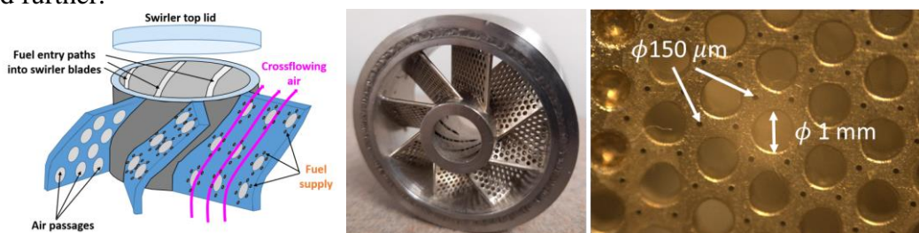
Figure 1: Schematic showing the fuel injection process by the MFIS swirler; Details of the swirler.
