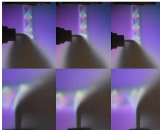
Figure 8: Shock structure interaction for varied injection location
