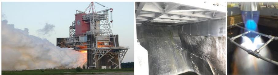
Figure 1: Left: Large scale test stand during test firing [2]; Middle: Damage caused to uncooled flame trench, NASA SSC. April 26, 2017; Right: Water spray ring used to cool Morpheus engine static tests [1]
