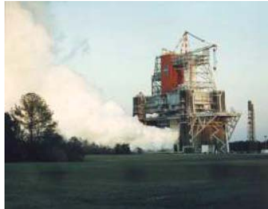
Figure 1: Space shuttle main engine undergoing test at the NASA Stennis B-1 test stand [1].
