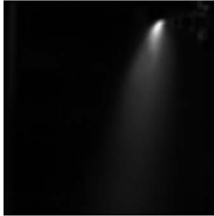
Figure 13: Averaged image after filtering for a case of 60 psi injection pressure as used to extract the penetration height.
