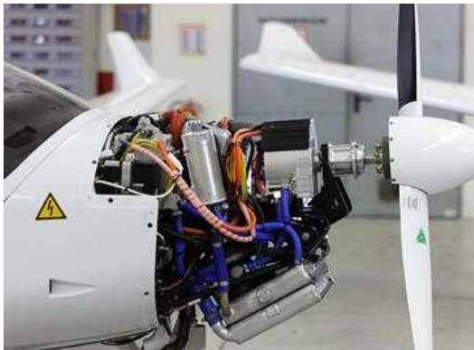
Figure 2 Siemens series hybrid drive system [3]
