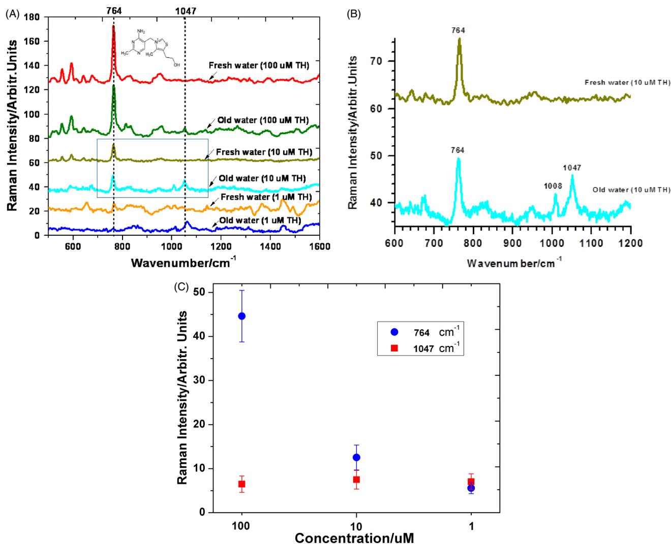
**Figure 2.** (A) SERS spectra of old and fresh thiamine hydrochloride (TH) solution of concentrations 1, 10, and 100  $\mu\text{M}$ . (B) Comparison of the SERS spectra for TH solution with the concentration of 10  $\mu\text{M}$  (zoomed in image for the cropped region on (A)). (C) Averaged intensities along with the standard deviations of the Raman peaks from old TH solution with three different concentrations for the wavenumbers 764 and 1047  $\text{cm}^{-1}$ .
