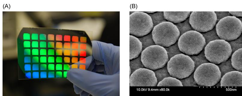
**Figure 1.** (A) Photograph of the nanodome SERS substrate. (B) SEM image of the surface of the nanodome SERS substrate with the perspective angle of 25°.
