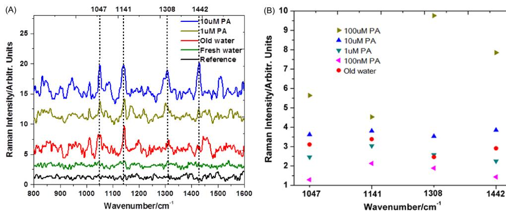
**Figure 4.** (A) SERS spectra of fresh water, old water, and phthalic acid (PA) solution with concentrations of 10 and 1  $\mu\text{M}$  and the bare substrate as reference. (B) Averaged peak intensities of old water and PA with different concentrations at 1047, 1141, 1308, and 1442  $\text{cm}^{-1}$ .
