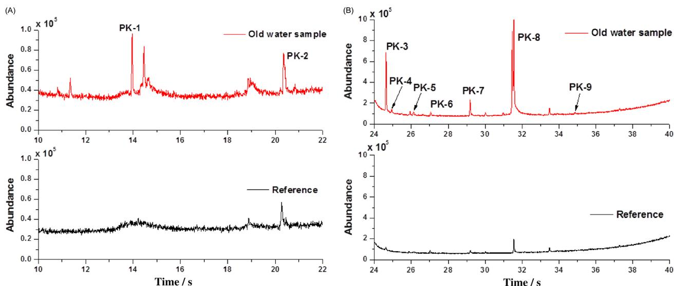
**Figure 3.** (A) GC-MS spectra of old water showing the two peaks corresponding to contaminants. The details of the contaminants are given in Supporting Information. (B) GC-MS spectra of old water showing more peaks at larger retention time corresponding to contaminants.
