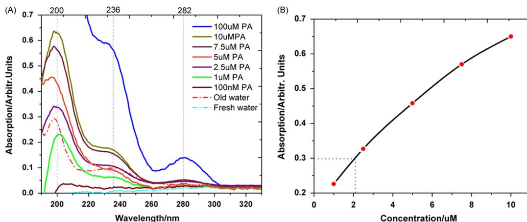
**Figure 5.** (A) UV absorption spectra for fresh water, old water, and phthalic acid (PA) solution with concentrations of 100 nM and 1, 2.5, 5, 7.5, 10, and 100  $\mu\text{M}$ . (B) Curve-fitting to the absorbance at the wavelength peak around 200 nm on (A) for PA with concentrations of 1, 2.5, 5, 7.5, and 10  $\mu\text{M}$ . The dotted line indicates the peak height for old water and its corresponding estimated concentration.
