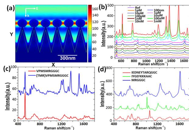
FIG. 3. (Color online) (a) 2D FEM simulation of electric field distribution on black silver. (b) SERS of R6g with different concentrations. (c) SERS of 100 nM peptides of the same sequence with and without TMR label. (d) SERS of 100 nM unlabeled peptides with three different sequences.
