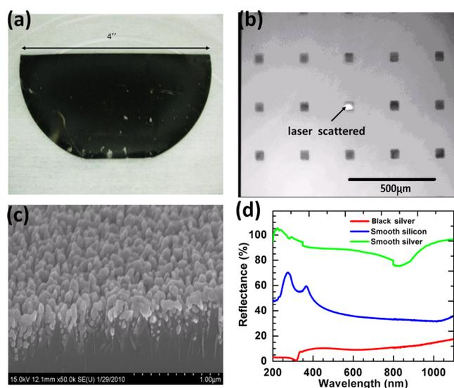
FIG. 1. (Color online) (a) Photograph of 4" black silicon wafer. (b) Photograph of square array patterned black silver. The shining spot is induced by laser. (c) Cross section SEM image of black silver substrate. (d) Reflectance spectra of black silver, smooth silver, and smooth silicon.
