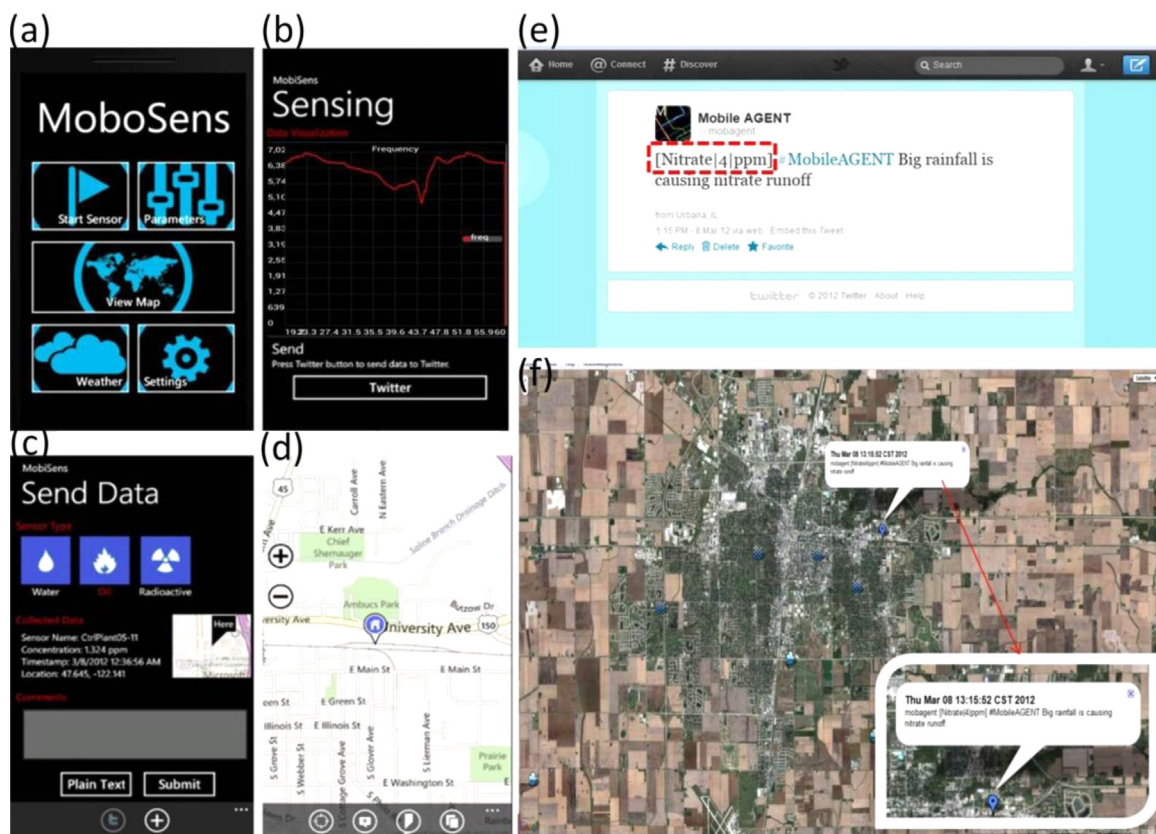
Fig. 7. User interface and network connection of MoboSens app. (a) Front page of the app. (b) Testing results plotted on the phone screen. (c) Interface showing the ability to input user “metadata”, along with the ability to pull publicly available data (e.g. USGS weather data) and showing them in one map. (d) Bing map interface with the current location of experiment shown on the map. (e) Message posted on Twitter website through the MoboSens platform. (f) Satellite view of recently posted data.
