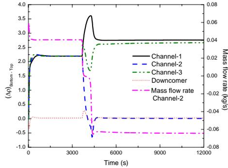
Fig. 4: Density variation at different Channels (Case-1)
