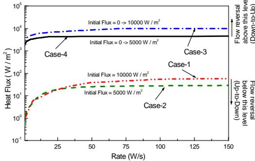
Fig.16: Flow reversal power level depending upon operation procedure at different power.
