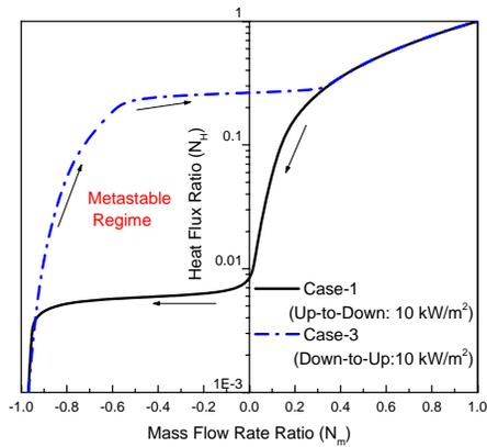
Fig. 18: Non-Dimensional Heat Flux Ratio ( $N_H$ ) for initial heat flux of  $10 \text{ kW/m}^2$  (Case-1 & 3)
