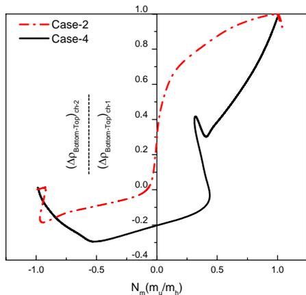
Fig. 19: Density difference ratio between Initially unheated and heated channel for initial heat flux of  $5 \text{ kW/m}^2$  (Case-2 & 4)
