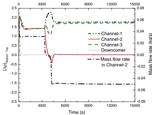
Fig. 7: Density difference between the bottom and top of different channels (Case-2)
