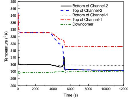
Fig. 3: Temperature variation at different Channels (Case-1)
