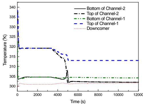
Fig. 6: Temperature variation at different Channels (Case-2)
