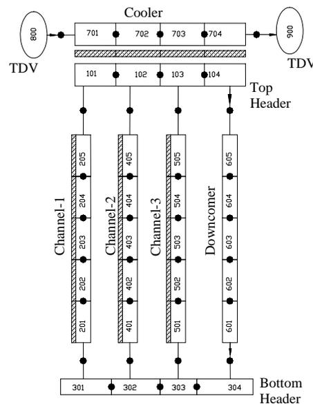
Fig.2: Nodalisation scheme for the natural circulation loop
