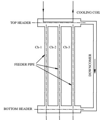
Fig.1: Schematic of the natural circulation loop
