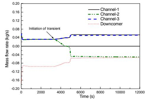
Fig. 9: Mass flow rate variations at different channels (Case-2)
