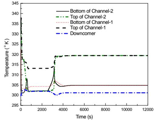
Fig.13: Temperature variation at different Channels (Case-4)
