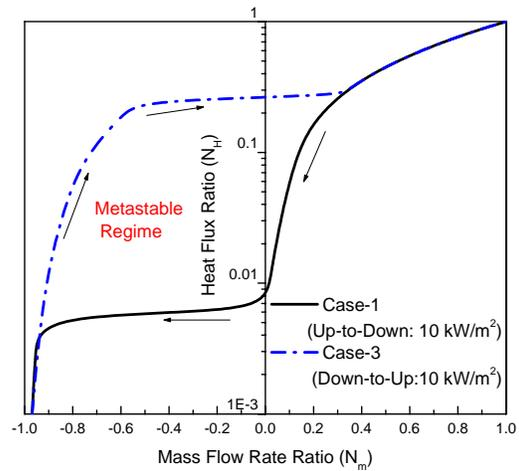
Fig. 13: Hysteresis effect during steady state in parallel channel natural circulation system
