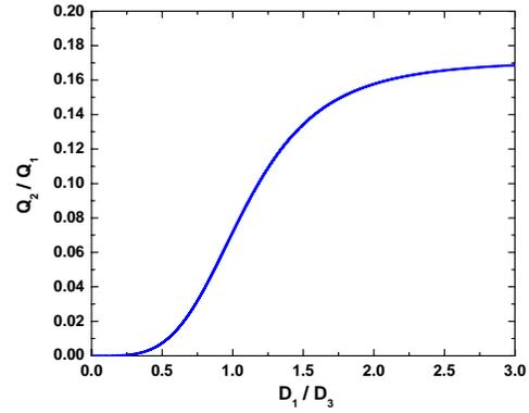
Fig. 6: Variation of non-dimensional power with high powered channel diameter
