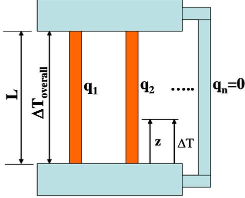
Fig. 1: Schematic of Parallel Channel Natural Circulation Loop
