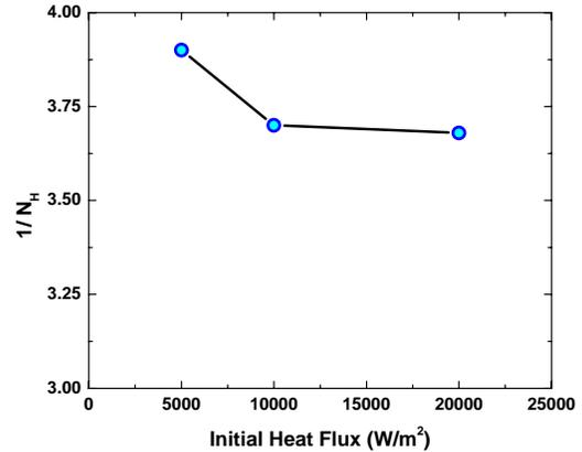
Fig. 16: Effect of initial heat flux values on  $1/N_H$
