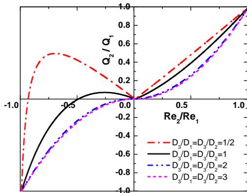
Fig. 5: Effect of adiabatic channel diameter on metastable regime
