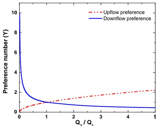
Fig. 2: Variation of preference number with non-dimensional power ratio
