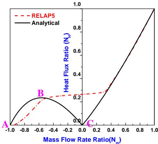
Fig. 12: Comparison of analytical and RELAP5 result
