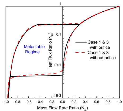
Fig. 14: Effect of orifice on the metastable regime
