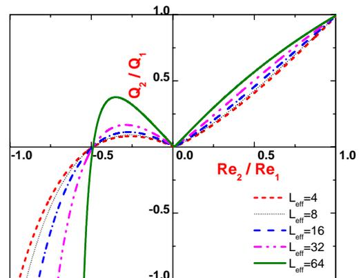
Fig. 8: Effect of loss coefficient on metastable regime
