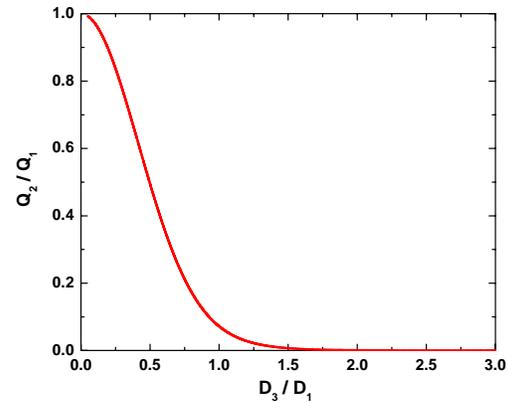
Fig. 7: Variation of non-dimensional power with adiabatic channel diameter
