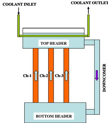
Fig. 9: Schematic of loop analyzed with RELAP5
