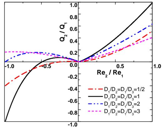
Fig. 3: Effect of high-powered channel diameter on metastable regime
