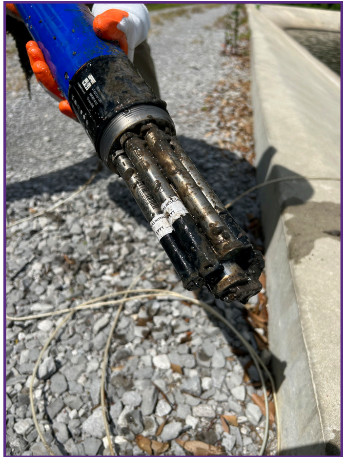
Water quality sondes have the capability to be submerged for long periods of time and monitor data in various time intervals using optical sensors. Photo by M.P. Hayes
