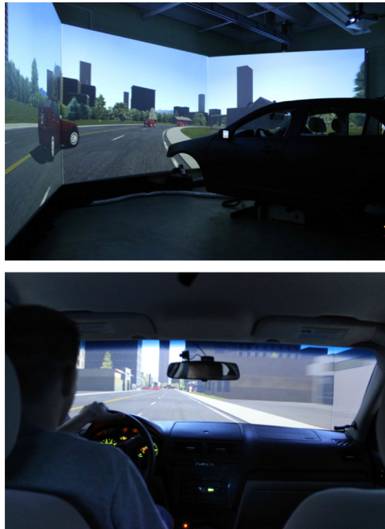
Fig. 1. View of Realtime Technologies Inc. Driving simulator from outside of the car (top). View of Realtime Technologies Inc. Driving simulator from inside of the car (bottom). Note that there were no other cars on the roadway in the current experiment. These images are meant to show the layout of the simulator. For examples of the simulated driving in the current study, see Fig. 2.
